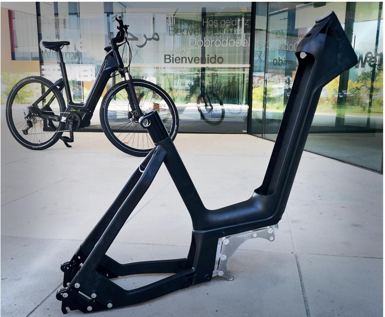
Flooded with water: the new generation of e-bike frames is manufactured by the WAIM process. © Engel Austria GmbH
