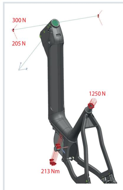
**Fig. 3.** Different loads acting on the cycle frame complement each other to form the load case. © SimpaTec
